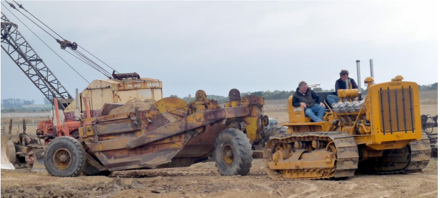
The Hutchings D8V8 takes off with a load, after a helping hand behind the scraper
