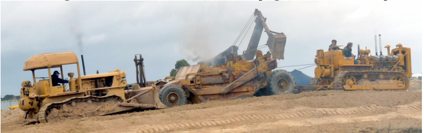
The Hutchings D8V8 takes off with a load, after a helping hand behind the scraper
