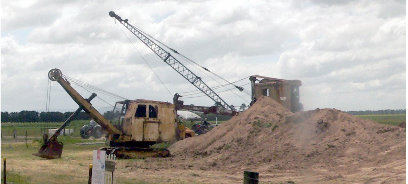
A Jaques J15 rigged as a face shovel is dwarfed by a 19RB Ruston Bucyrus Drag line
