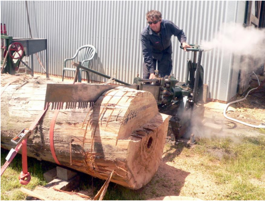
Darren Guy sets up the steam drag saw and tests the steam whistle above his immaculately manifolded boilerhouse shown below. This display of kerosene pressure lamps reflects earlier days.
