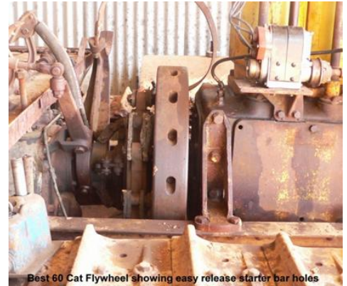
Best 60 Cat Flywheel showing easy release starter bar holes
