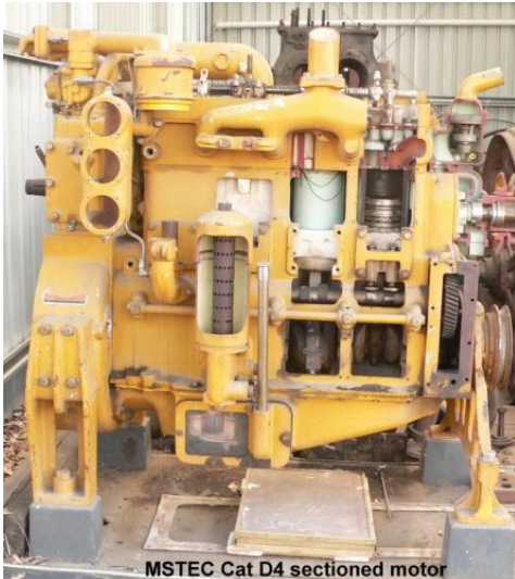
MSTEC Cat D4 sectioned motor
