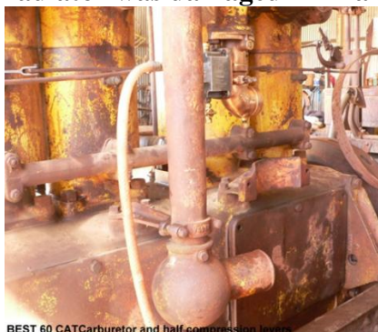
BEST 60 CATCarburetor and half-compression levers
