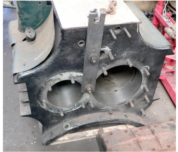
Boring bar close up and a look at the bore after the job is complete ( the LP Cylinder was sleeved)
