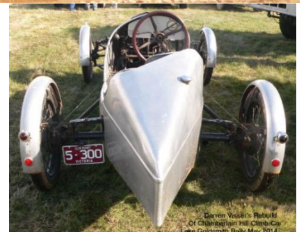
Darren Visser and Son Luke take a spin in this rebuild of Chamberlains successful 1920 style Hill climb car. The motor is a from an Indian Motor bike, and the travelling mechanics seat is low comfort
