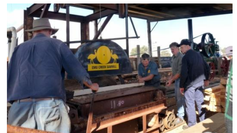
Steam was not left out of the log handling demonstrations, here Scobie Bros go back to an earlier era when steam provided the motive force to move and mill timber. Steam provide the power for the Smith's Emu Creek Mill/ For this rally a portable was in action
