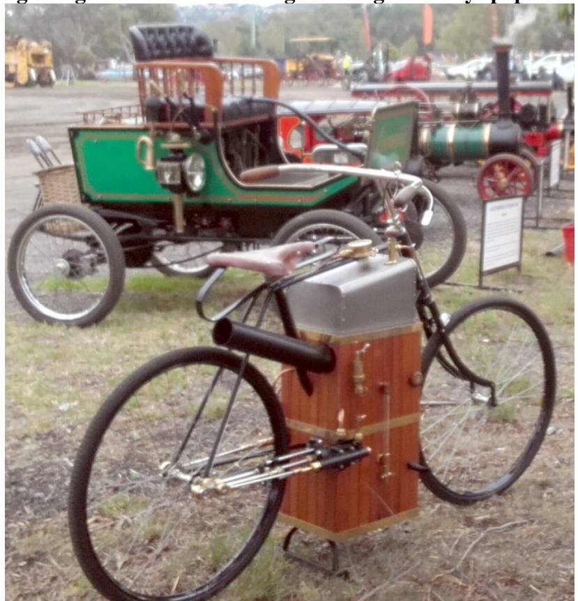
. This Replica of an 1896 roper Steam powered Motor Bike was an attention getter with its external piston and valve gear
