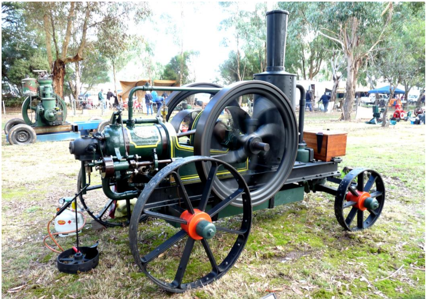
This immaculate Blackstone Oil Engine needed a bit of extra heat to idle.
