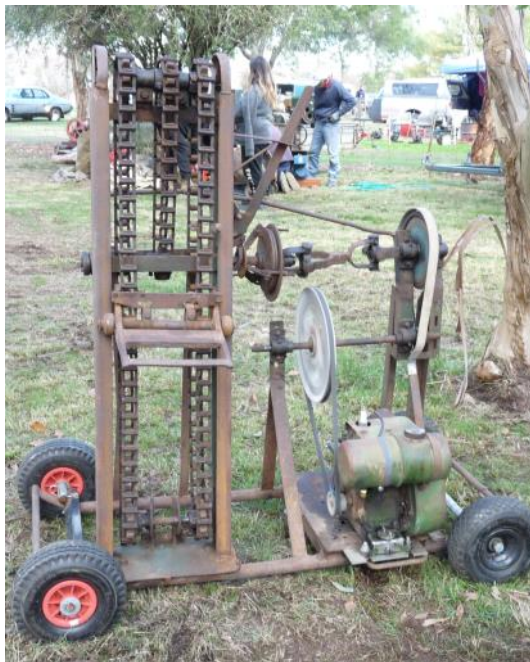
Left above is a powered vintage bag lifter from the days before Reynolds chains. And on the right above this pair has made an early start for the November rally for British tractors. They really are a compact crawler and this one looks near "New".
