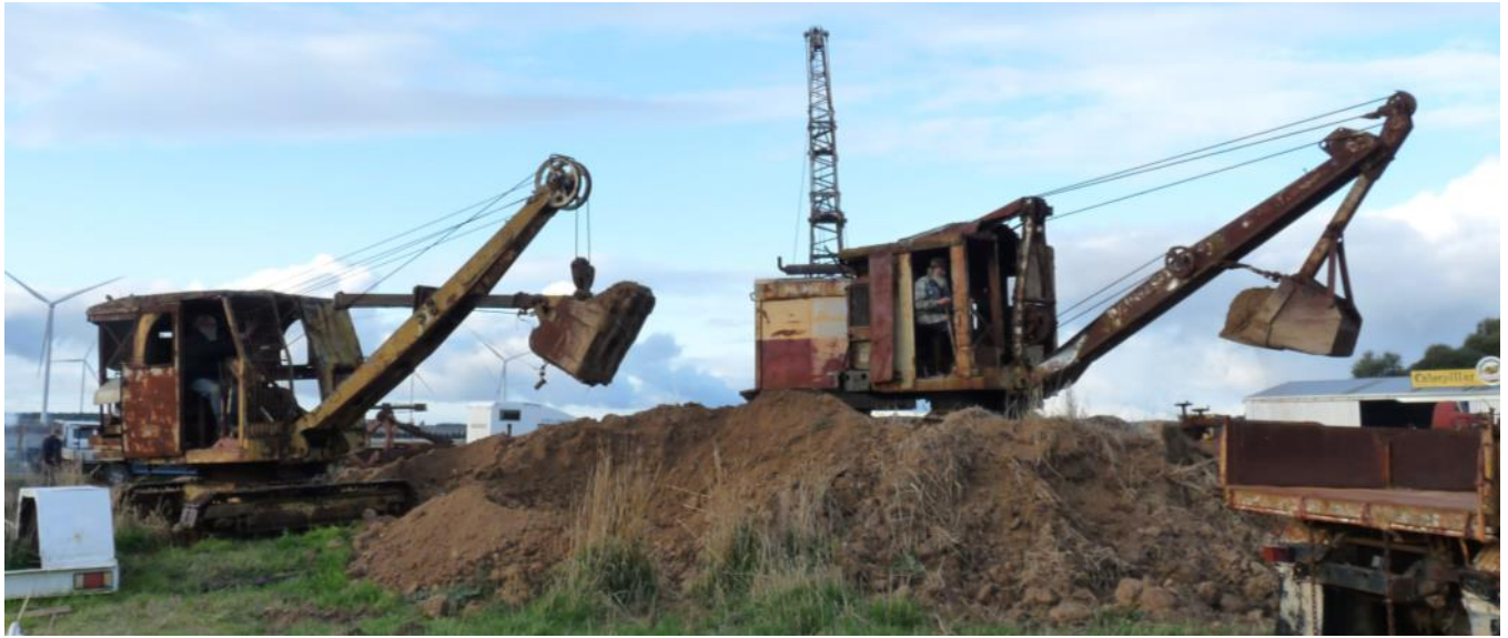
Left above, The Jacques J15 face Shovel gets some back acting competition while the Ruston Drag line is hidden away in the background.
