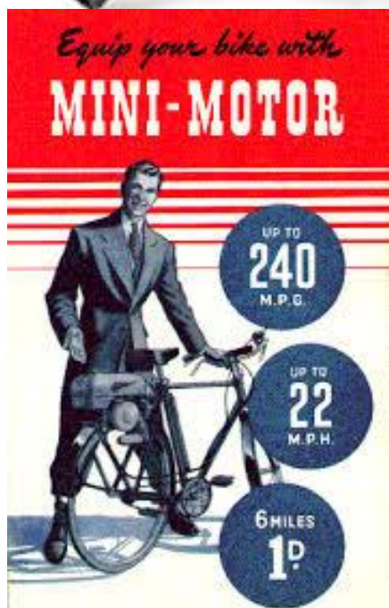
On the right is the Trojan mini motor 2 stroke engine as a power booster behind the seat of a push bike. Vincenti developed these 49cc engines in Italy in 1946, and Trojan, who made 2 stroke cars in the UK made the in Croydon from 1947 to 1957. These machines were quite popular here and ever now and then we see one at a rally. They drive the rear wheel directly using a friction wheel on the tyre.
