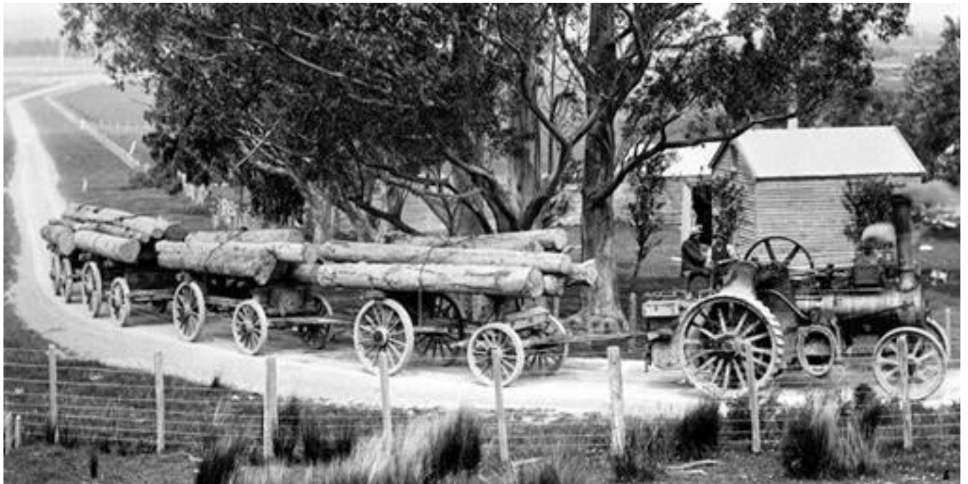
Road Trains were in use very early. This set of 4 towed carriages makes a great sight in a bush setting. Horses could not compete with Traction Engines which only needed 2 operators compared to 4 who would have been needed to man the wagons.
