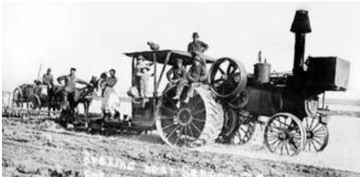
These American Traction Engines were used to direct ploughing the hard Prairie soil.
