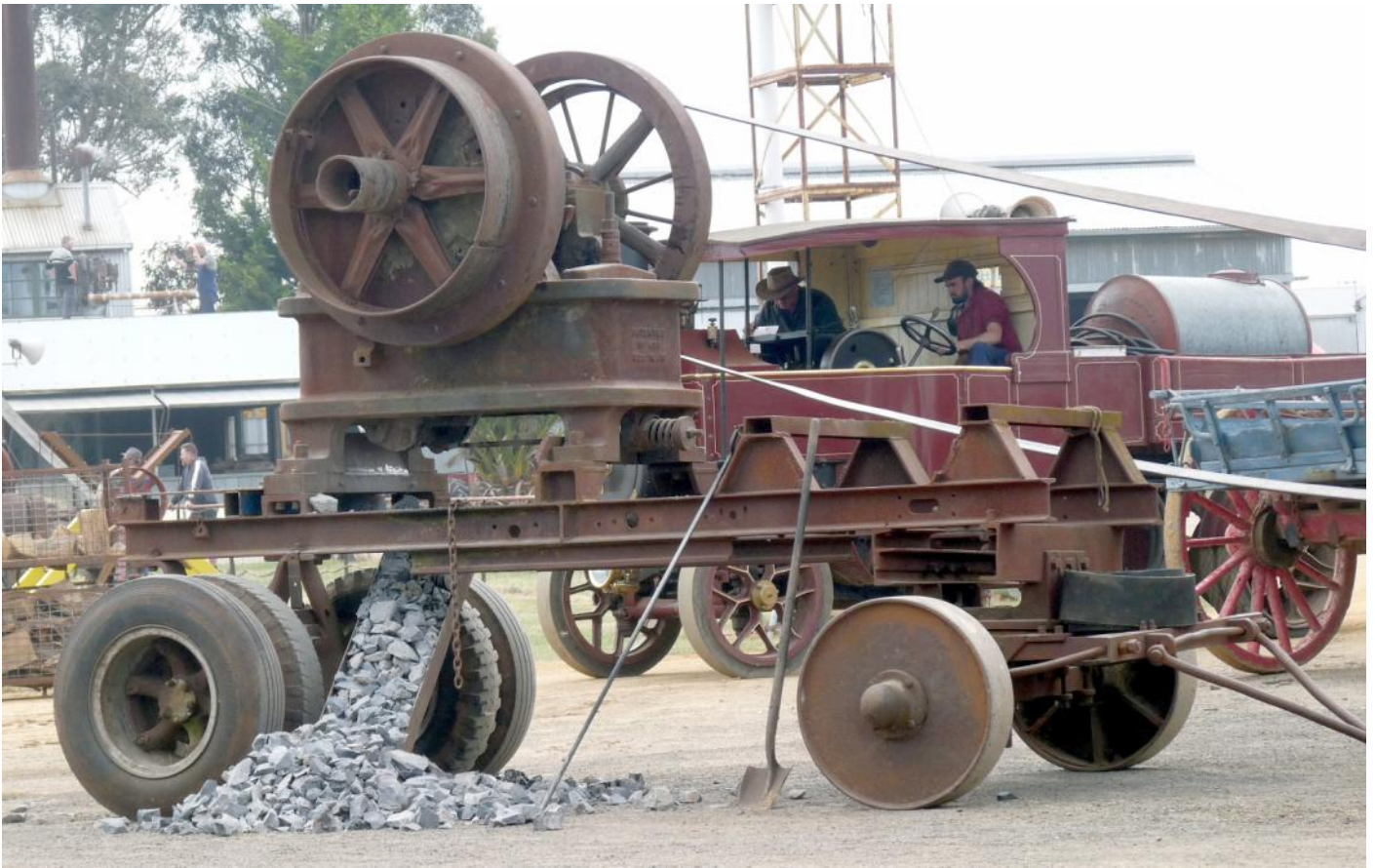
A second portable stone crusher was in action, with a Foden Steam Wagon behind which had been used to move the stone (top right picture on the last page). Graders were not the only Malcom Moore machinery that were based on Fordson Tractors. This cable operated mechanical loader was another reminder of pre-hydraulic earthmoving machinery ( below left ). Below right, this Tar heat-
