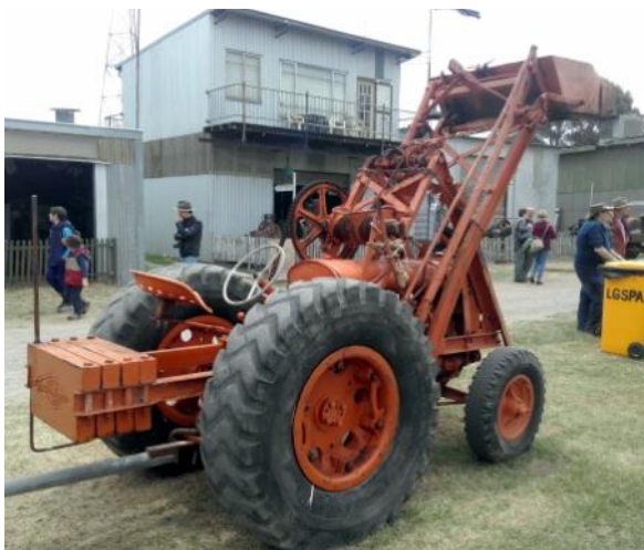
A second portable stone crusher was in action, with a Foden Steam Wagon behind which had been used to move the stone (top right picture on the last page). Graders were not the only Malcom Moore machinery that were based on Fordson Tractors. This cable operated mechanical loader was another reminder of pre-hydraulic earthmoving machinery ( below left ). Below right, this Tar heat-
