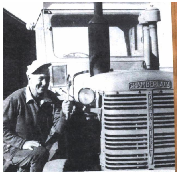
● BOB Hathway with the Super 70 Chamberlain that has more than 27,000 hours on the clock — and still running like the day it was bought.
