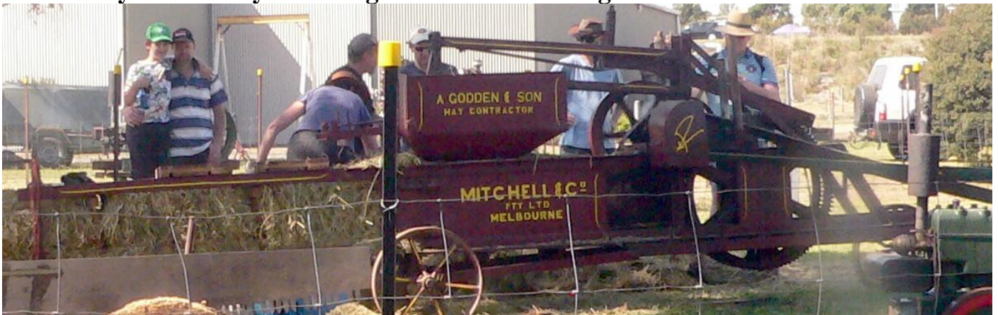
Square bales were made in this hand fed, belt driven Mitchell & Co. hay press,
